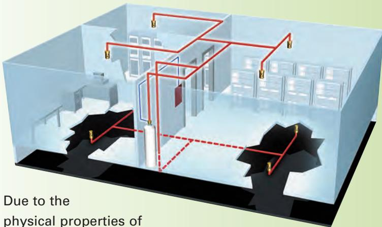
Due to the physical properties of Dupont's FE-25 and the superior performance of Fike's fast-acting rupture disc valve assembly, **ECARO-25** can work with your existing Halon pipe network – just replace the nozzles and containers. With **ECARO-25**, you can easily transform your old Halon 1301 fire suppression system into an effective, environmentally-sound clean agent system, with minimal system modifications.
