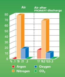
Reduced oxygen levels will not sustain a combustion reaction, but are acceptable for human exposure over a short period of time.
